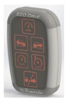
Eco Driving means smarter and more fuel-efficient driving. It can reduce fuel use and  $CO_2$ emissions by up to 20%. The Eco Driving monitor attached to the vehicle's onboard computer informs the driver of every non-economic move, and sets benchmarks for driving efficiency. This eco driving intelligence is logged into an online system and can be later analysed.
